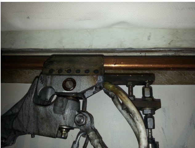
Pantograph converted to spray head
