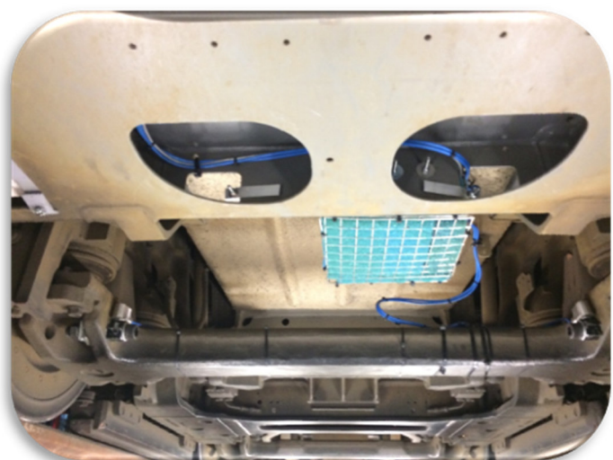
Device installed in vehicle bogie
