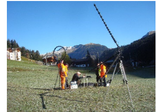
Noise measurements with acoustic cameras.
