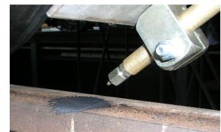
The correct adjustment of the nozzles is important for an effective lubrication system.
